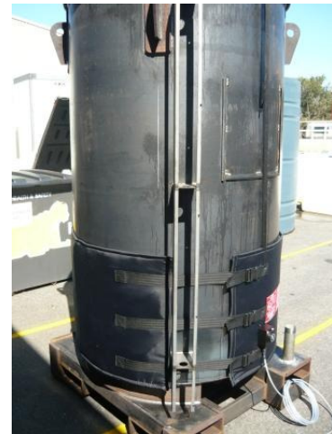
Blanket has straps to join ends together under gauge
