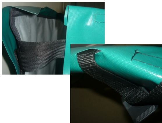
Over-cover folds over the top of the heater jacket and around the vertical straps to give some dust and wet protection.
