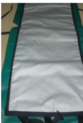
Inside surface of heater blanket showing overlapping PVC cover.
