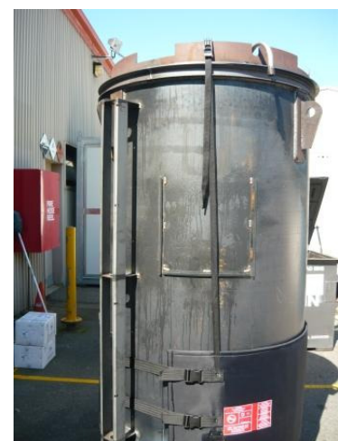
Transtainer RTM-145 showing vertical support strap. This is hooked on and the jacket is walked around the container.
