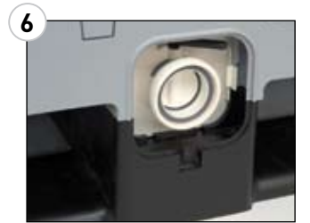
6 BOTTOM DISCHARGE OPENING The bottom discharge opening is located below the drop door and positioned below the inside bottom level to ensure maximum discharge performance without manual assistance. A range of glands and valves are available to fit the outlet. A tamper evident cap is used to cover the outlet.
