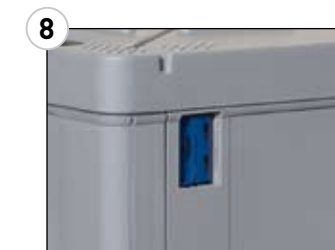
8 WALL LOCKING CLIPS The clips prevent unintended folding of the container. By moving the clips inwards the walls can easily be folded.
