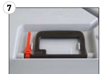
7 TAMPER EVIDENT LOCKING DEVICE The (4x) locking device is a strong and durable all plastic design. It is simply operated to open or close through a lift and slide motion. To secure the locking a seal ensures the tamper evidence.
