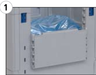
1 DROP DOOR The access door is opened to facilitate the liner installation
