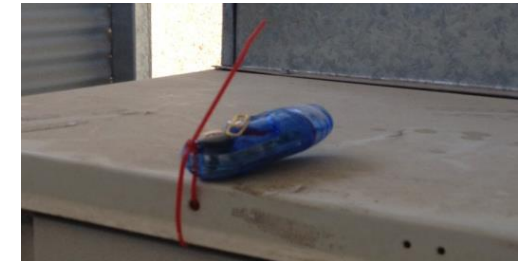
Fig. 4 Air on condenser data logger mounted in centre of mesh
