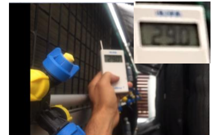
Fig. 5 Hanna probe - ambient of 32.2 C and the air on coil temp of 29C
