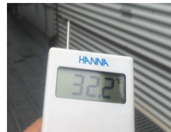
Fig. 5 Hanna probe - ambient of 32.2 C and the air on coil temp of 29C
