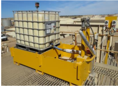
Lubrication tanks and pumps are supplied on skids, or in stand alone shipping containers
